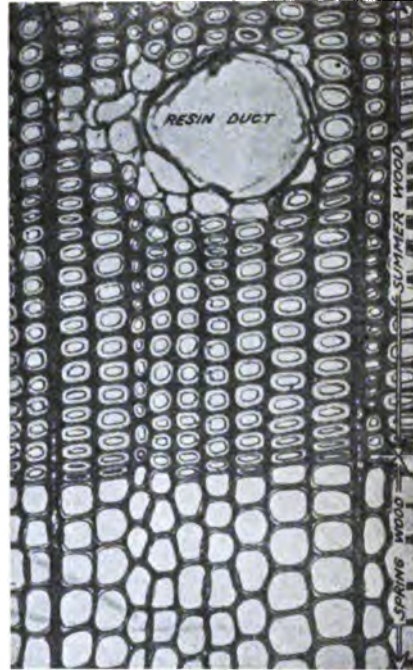
FIG. 4. — Transverse Section of Shortleaf Pine, Showing Resin Duct. (Magnification 125 diameters.) (Bull. 101, U. S. For. Ser.)
